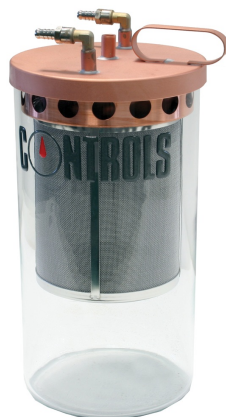
Wire basket in the jar with supporting ring and metal condenser
